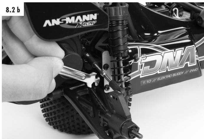
Negative camber on the front wheels increases the cornering forces of the wheels when cornering. The steering is more direct, and more responsive.
